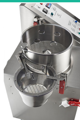
Production spheronizer discharge system
