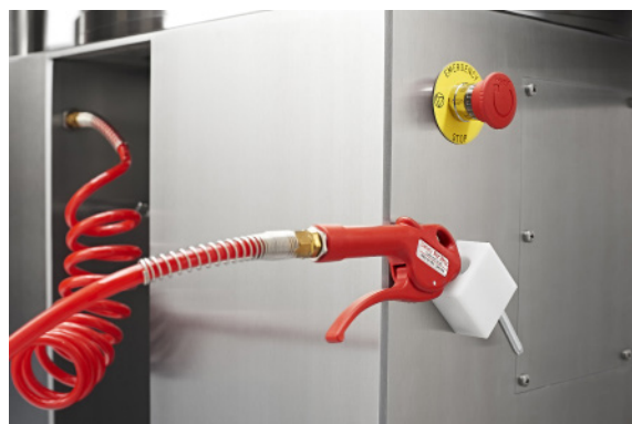
"Clean without stopping" spheronizer air blast system
